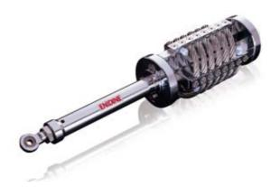
WEAR™ (Wire Energy Absorbing Rope) pipe restraints are uniquely packaged wire rope isolators designed to protect structures from steady state vibration and isolate them from seismic and dynamic loads. These new generation energy absorbing restraints feature simple construction. There are no oils, seals or complex moving parts required to perform their function. The design has eliminated the problems often associated with hydraulic or mechanical restraints which are complex and prone to failure.
